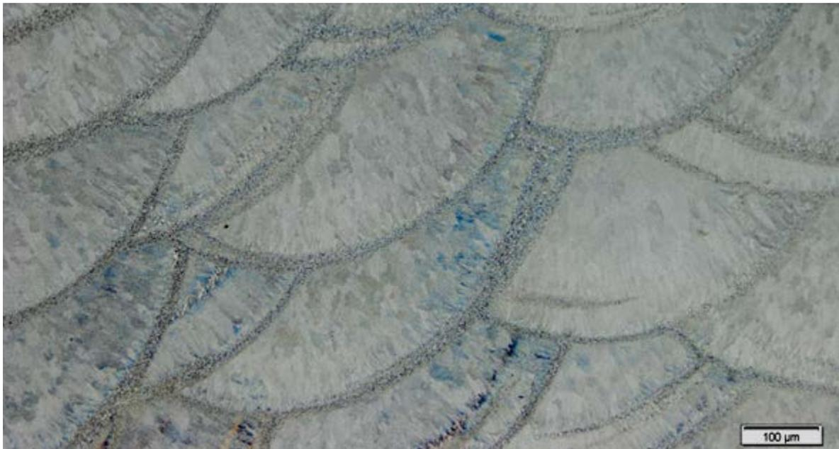
Figure: Microstructure overview in a slightly hyper-eutectic Fe-Fe<sub>2</sub>Ti alloy processed by Laser Metal Deposition.
